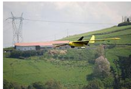
Figure 3.4: Fulmar UAV, developed by Aerovision for civilian applications.
