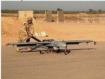
Figure 3.3 The RQ-7 Shadow is capable of delivering a 20 lb (9.1 kg) "Quick-MEDS"
