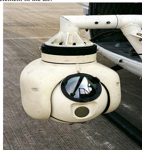
Figure 3.1: A forward looking infrared (FLIR) camera mounted on the side of an UAV
